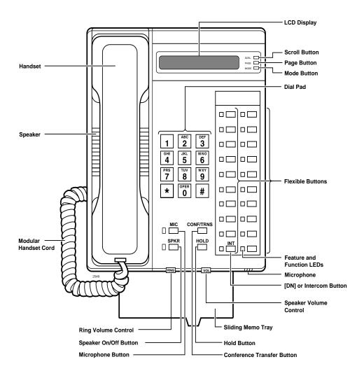
Figure 1 20-Button Electronic Key Telephone with LCD
